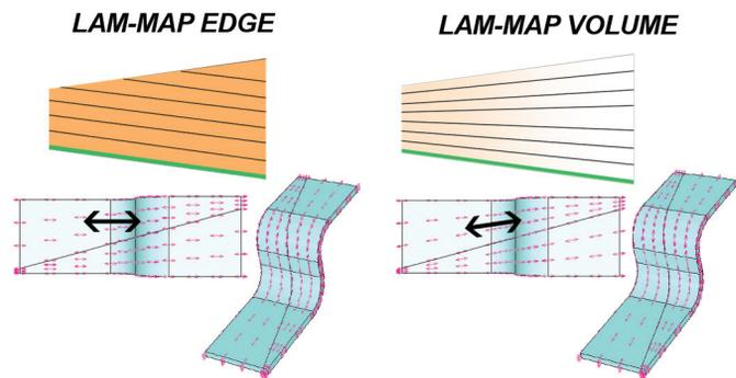
These options allow modeling injection molded parts that include cut fibers which orient themselves with the mold. StressCheck® allows you to display arrows representing the principal direction for laminates, which is particularly useful when visualizing the ply angle orientations.
