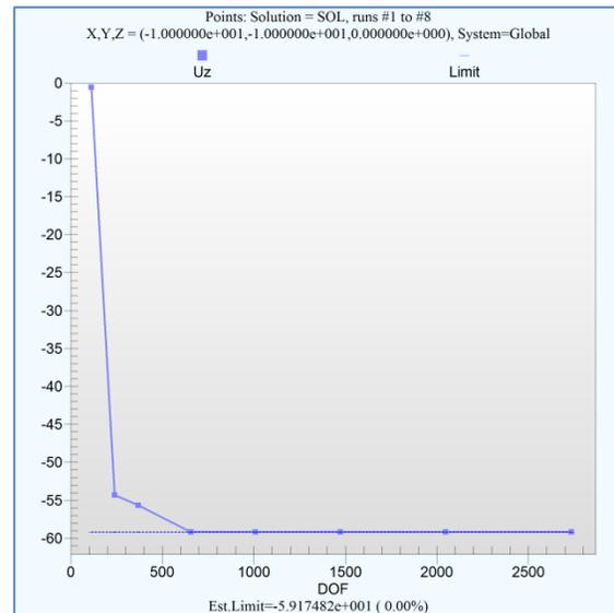
Figure 2: Convergence of displacement using 3D elements with antisymmetry constraints (verification)
