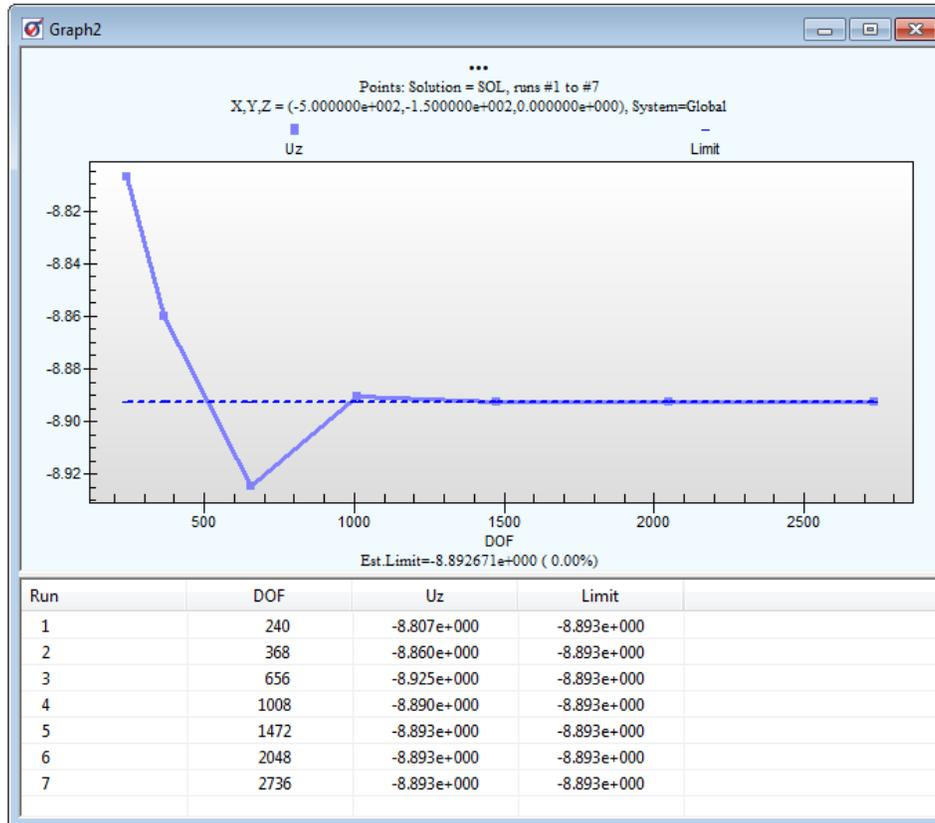
Figure 7: Convergence of displacement
