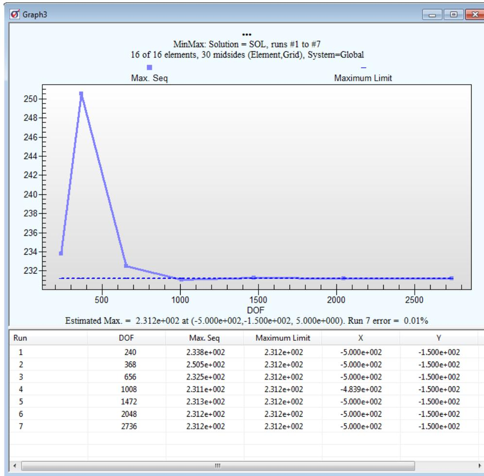
Figure 8: Convergence of von Mises stress
