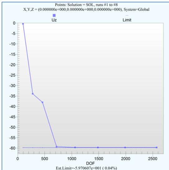
Figure 1: Convergence of displacement for plate elements with simple supports (verification)
