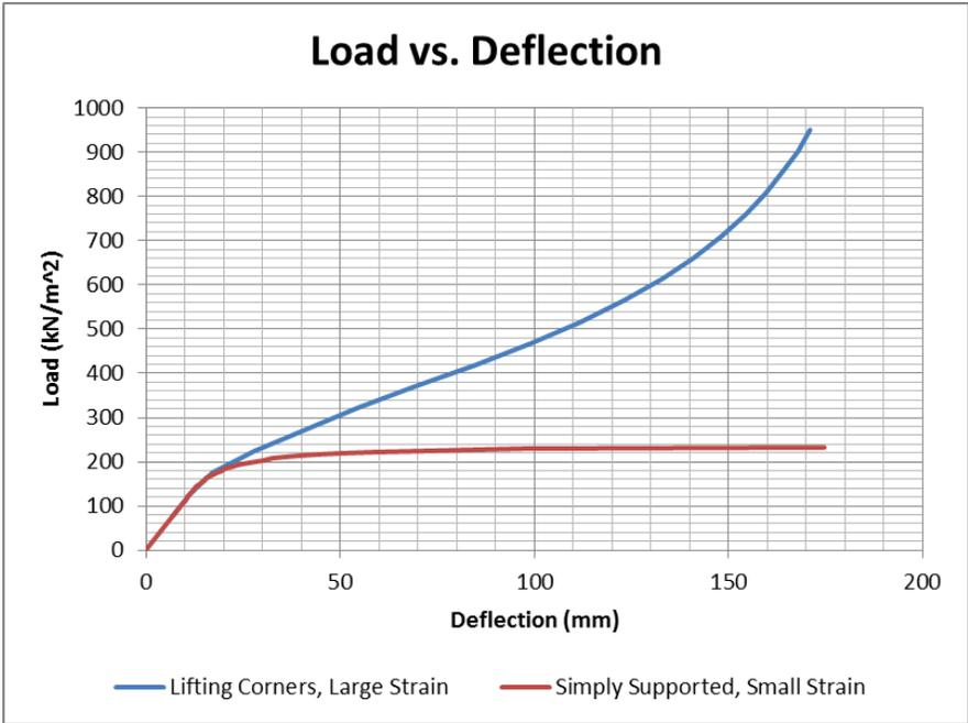
Figure 10: Comparison of load vs. deflection for lifting corners and large strain elasticity and the previous results
