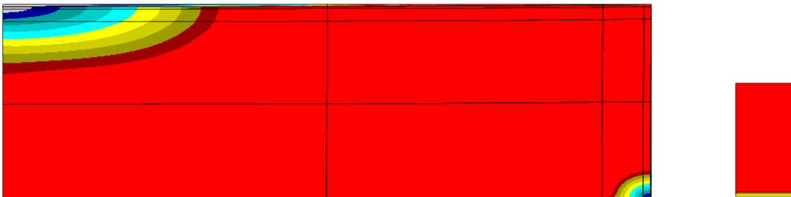
The final collapse load is approximately 230 kN/m<sup>2</sup>, which is close to the value given by Roark. Why the difference? The FEM solution presented is a higher-order model than the Roark solution which was likely obtained with an analytical approximation. As such, the Roark solution is expected to be conservative.
