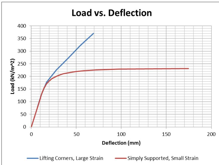
Figure 12: Comparison of load vs. deflection for lifting corners and large strain elasticity and the previous results
