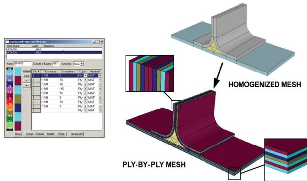
Material directions can reference Cartesian or cylindrical coordinate systems. However, for many practical problems, a general curvature approach is needed. StressCheck® has two unique capabilities allowing you to align the material properties with the curvature of an element with the Lam-MapEdge and Lam-MapVolume options.
